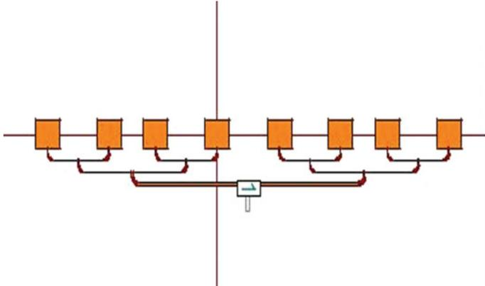
**Fig. 1** Array of  $8 \times 1$  microstrip square antenna
